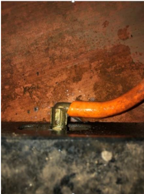
Figure 2. No soap bubbles at the missing clamp, indicating no leak.
