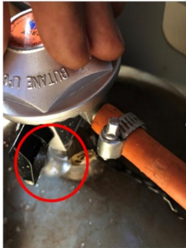
Figure 1. Soap bubbles show location of leak at the gas cylinder seal.
